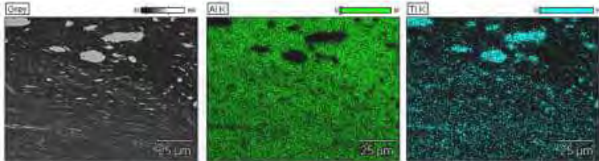
Fig. 6. EDX maps of the Al-Ti sample processed for 50 turns.
