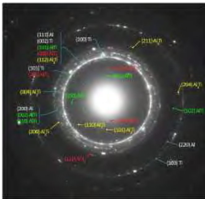
Fig. 9. SAED pattern showing presence of several intermetallic phases from the Al-Ti system.
